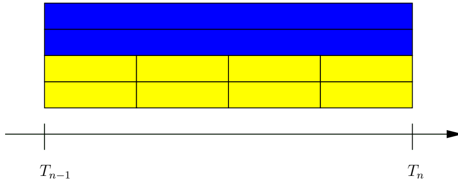
FIGURE 4. A time slab with N_K = N_k = 2 and multi-adaptive efficiency index \mu = 16/10 = 1.6
